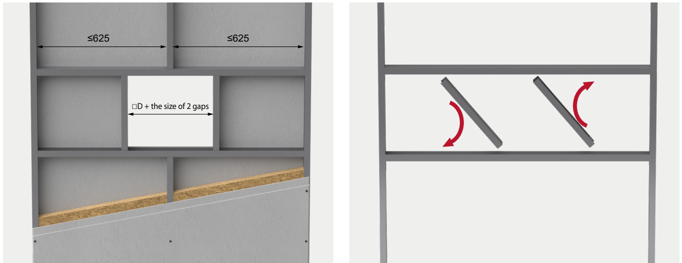
Installation opening reinforcement in the flexible wall
