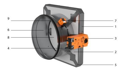
1 – metal collar, 2 – calcium-silicate fire-resistant flange, 3 – 24V / 230V actuator, 4 – connecting wires, 5 – installation holes, 6 – metal casing, 7 – 72 °C thermosensor, 8 – calcium-silicate blade, 9 – casing insulating rubber
