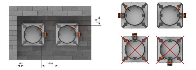
6. Selection of the montage fastening shall be conducted depending on type of the supporting construction (e.g., aerated concrete, drywall, masonry wall) and also based on the weight of the damper:
