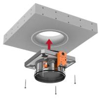
3. Both positions of the fire damper below or above the ceiling panel are permitted.
