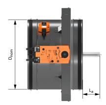
3. Fire dampers are originally delivered with closed blade. **If a fire damper has been installed with an open blade, this may cause incomplete closing of the blade or even damage!** Blade position can be controlled by referring to marks located on the actuator's casing: 0° is equivalent to Closed position, 90° is equivalent to Open position:
