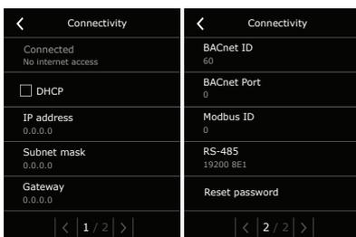
**Remote control** – settings needed to access the unit remotely.
