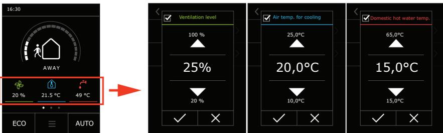
In this window you can temporarily disable individual part of the unit (ventilation, hot water production, underfloor heating) by unchecking the box next to the setting.
