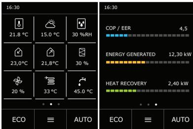
If you want to monitor other parameters that are not displayed in this window, press and hold for 5 seconds the parameter in place of which you want to see a different one. This will take you to a settings window where you could choose data to display (approx. 20 different parameters).
