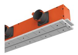
**PROFILE 600** model diffuser is designed for plasterboard ceilings / walls, connecting to a 75 mm flexible duct system, contains a balancing valve. The design is compact, requiring just 17 cm of installation depth.
