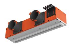
**SINGLE 500** model diffuser is designed for plasterboard ceilings / walls, connecting to a 75 mm flexible duct system, contains a balancing valve & needs only 12 cm for installation.
