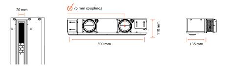
LINEO 500 diffusers are designed for flexible plastic duct systems with a 75 mm diameter. They can be mounted vertically or horizontally and feature a compact design, requiring only 12 cm of installation space, making them ideal for saving space beneath plasterboard ceilings. They are also suitable for installation in 12 cm thick partition walls.
