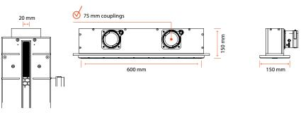
LINEO 600/75 PROFILE diffusers are designed for flexible plastic duct systems with a 75 mm diameter. They can be mounted vertically or horizontally and feature a compact design, requiring only 17 cm of installation space.
