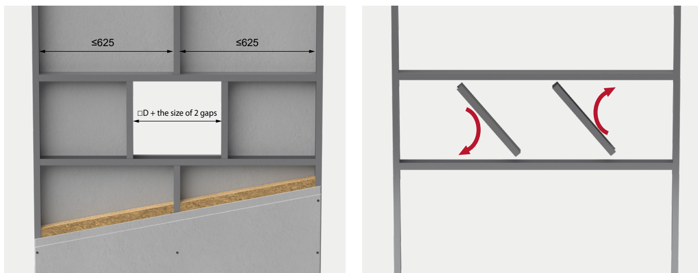
Installation opening reinforcement in the flexible wall
