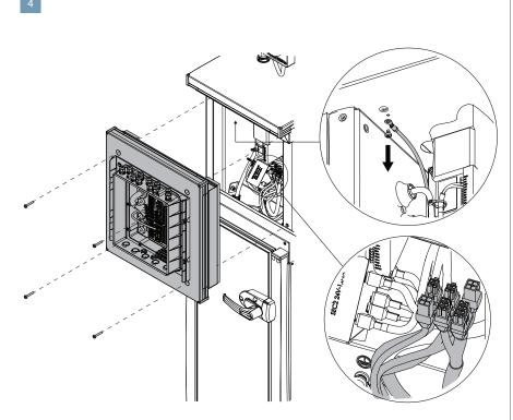
Loosen four screws at the corners of the automation panel. Carefully pull the panel to yourself and disconnect cable terminals on the back of the panel. Also disconnect the earthing cable fixed to the top panel of the section.
