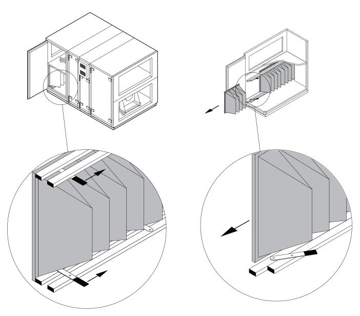
Fig. 4. Filter clamping device
