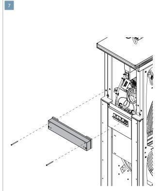
Loosen screws (2 pcs.) and remove the crossbar.
