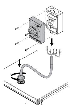
Disassemble the main circuit breaker box and disconnect the power cord. Unscrew the cable gland and pull the entire power cord inside the section.
