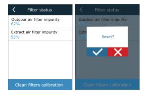
When replacing filters with filters from different manufacturers or different filtration class, calibration of clean filters is recommended. During calibration, the unit will operate at a maximum speed for a few minutes, measure the pressure difference upstream and downstream the filter and automatically determine the filtration class.
