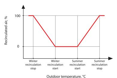
Fig. 3. REC function operation
