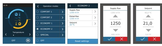
SPECIAL ventilation mode may also be used to disable heating/cooling and other functions. This saves energy when temperature and other ventilation parameters are less important (for example, at night, when the building is empty, when cooling devices can be turned off and will not be activated even when temperature exceeds the desired temperature during the day).
