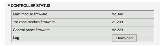
For detailed performance analysis, you may download a device logbook (Log) which contains weekly operation data. To open a logbook you will need a "Log plotter" app that you can download on the "Komfovent" website. This data can be useful in the event of a failure and may facilitate repair procedures, therefore, we recommend downloading an operation logbook and handing it over to the authorised service personnel.
