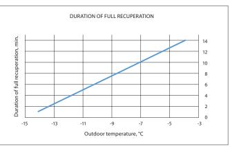
If outdoor temperature drops bellow -15  $^{\circ}$ C, full recuperation is not done and segments closing/opening intervals are the same.
