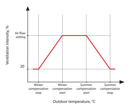
Fig. 2. OCV function operation
