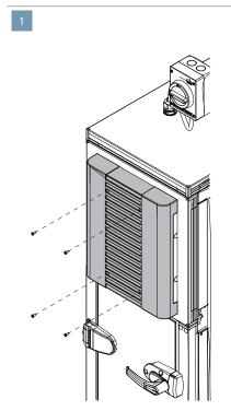
Loosen the screws on the automation box cover (4 pcs.).
