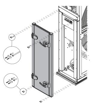
Loosen the screws holding the door struts (8 pcs.) and remove them together with the door.
