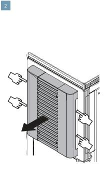
Press the indentations on the sides of the box and release the latches holding the cover. Press two latches on the same side of the box at the same time.
