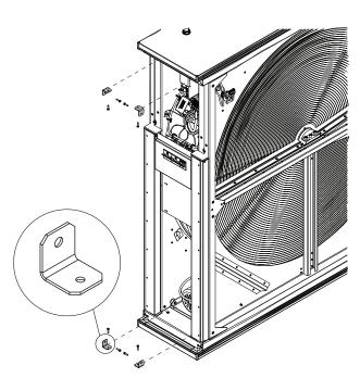
Unscrew the brackets at the corners that secure the rotor housing to the top and bottom of the section (brackets may not be used in smaller units).
