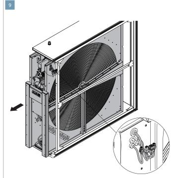
Disconnect cable connections from the filters, inspection or recirculation section side. Pull the rotor housing out of the section about 10cm. Pull the cable connections through the gap between the rotor housing and the fan section and disconnect them.
